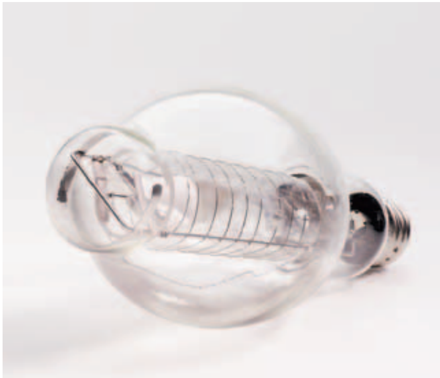
Few watts per sq. ft. are required with the pulse-start metal-halide fixtures, because increased light levels are assured through the life of the lamp.
