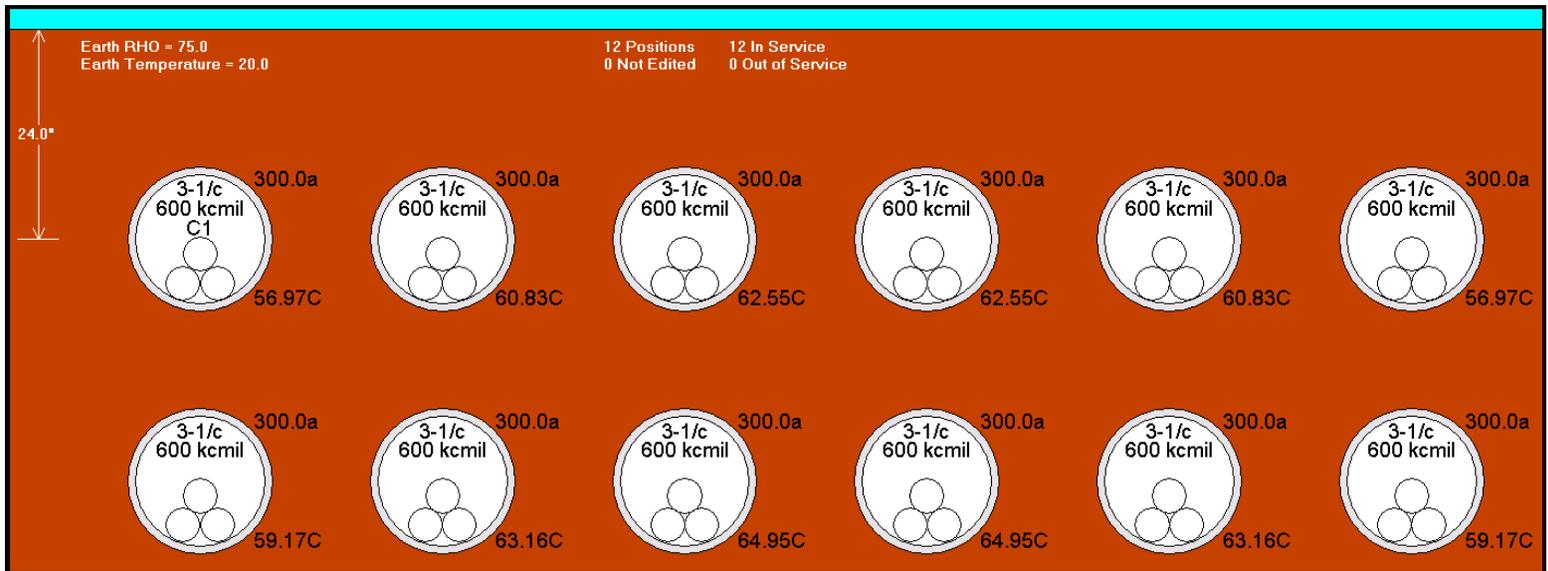
Additionally, these programs will calculate the total loss of energy due to heating and the voltage drop of the conductor. The energy wasted through the conductors due to heat loss can be a significant number and should be considered with any evaluation of these type of electrical duct banks.
