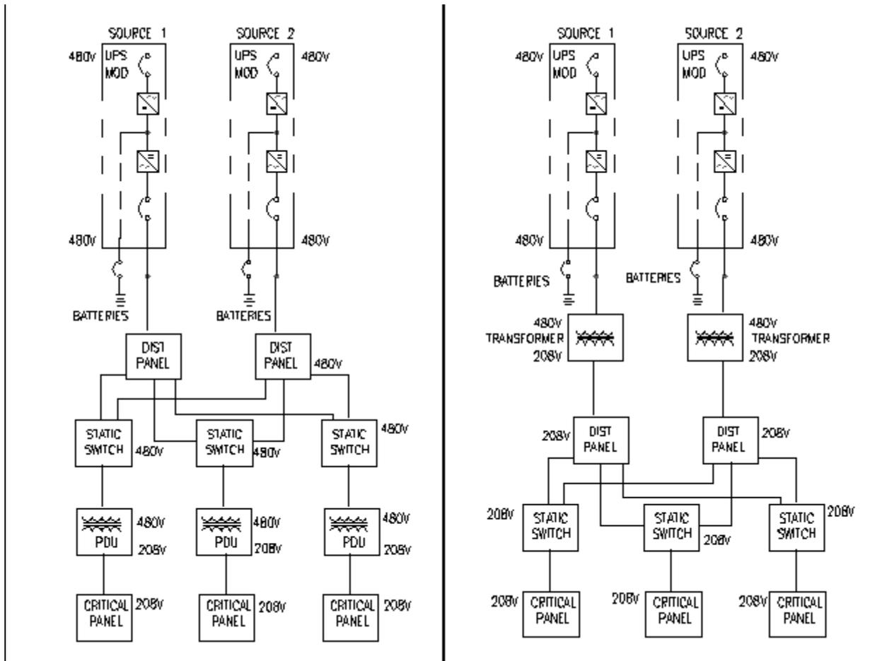
**Figure 3 - Electrical Distribution System**
