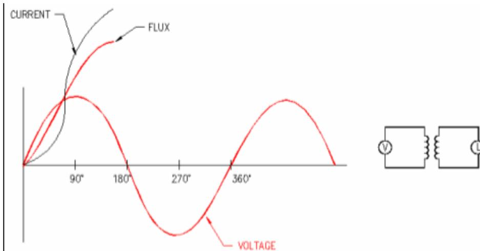
**Figure 1 - Transformer Flux and Inrush Current at Zero Voltage Crossing**
